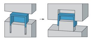
Using a core cavity, as shown, can be a cost-effective method of moulding tall walls and ribbed surfaces.
