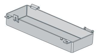
➤ This is an example of one half of a self-mating part, which fits together in either direction with its other half, building a "universal" part.
